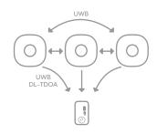
SATIets synchronize wirelessly with each other and provide UWB signals as broad cast for the TRACElet. The UWB signals work according to the downlink TDOA method and can be used by the TRACElet for positioning.
